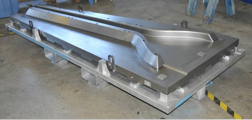
Draping mold AIRBUS HELICOPTER X4 (H160)
